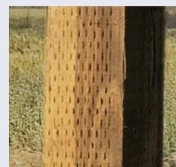
is a heartwood penetration requirement (*even for permeable species such as pine*). **Mechanical incising** of the surface is now used widely to help achieve the desired penetration.
